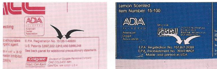
FIG. 4 Comparison of EPA Registration Numbers on disinfectants shows which packages contain identical formulations. Compare the group of numbers before and after the first hyphen or space. If they are identical, the formulations are identical. Ignore the numbers after the second hyphen or space. By U.S. law, all products claiming disinfection must have EPA registration displayed somewhere on the package label.
