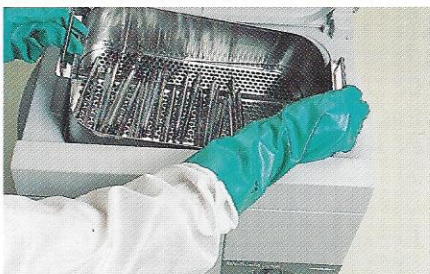
7b. Transfer instruments to a powerful ultrasonic cleaner and operate at least 1.5 minutes per instrument for loose instruments and at least 15 minutes total for instruments within a cassette, then rinse.
