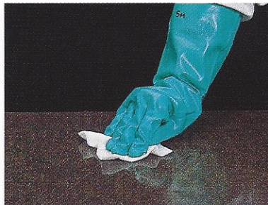
6e. Use second applicator to scrub the surfaces to remove visible debris.
